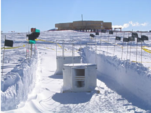
(a) Every IceTop station consists of two IceTop tanks. The picture shows the two tanks of station 21 before refilling.
