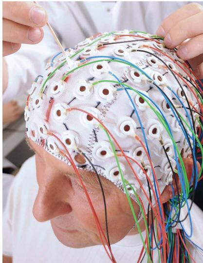
Figure 2.7: An electroencephalography cap with 128 electrodes
