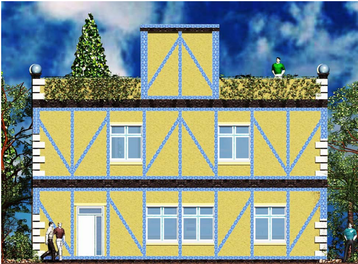
Figure 5-3: Front view of a family house with different types of panels [Courtesy: N. Nasserian]
