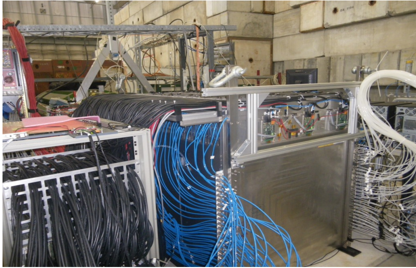
Figure 3.19: Picture of the SDHCAL technological prototype during the test beam at SPS, CERN 2012 [48].
