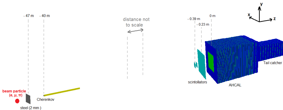
Figure 6.17: Sketch of the simulated beamline. The dimensions are not to scale. Positions: AHCAL at 0 m, beam particles at - 50 m and the additional steel material at - 47 m.
