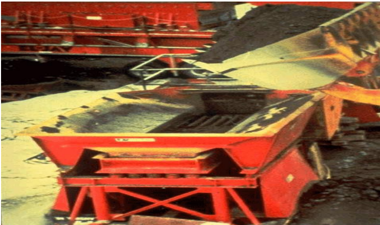
Fig. 17: Reclaimed asphalt pavement (RAP) crusher ( fhwa.dot.gov/pavement/recycling/98042/05.cfm last accessed on 26.09.2018)
