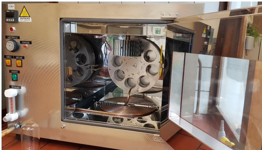
Fig. 7: RTFOT ageing apparatus (source: BestLab at the University of Wuppertal).
