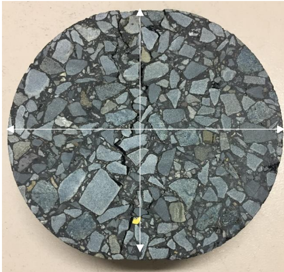
Fig. 66: Failure shape and path of different mixes, (a) SMA 11 S and (b) AC 22 T S mix
