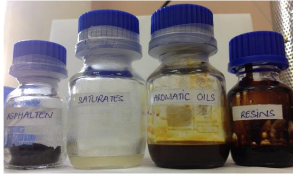
Fig. 2: Chemical compositions of asphalt molecule ( http://bmt-rnd.vn/cong-trinh/sara-fraction-and-colloidal-structure/?lang=en , last access 26.12.2018).
