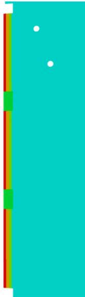
Figure 6.2: Geometry of the two-dimensional model of an IEC 60099-4 surge arrester. The air region is colored in turquoise. The components of the surge arrester are colored in red, green, and orange. Areas, where the surge arrester pierces through the air plane are colored in white.
