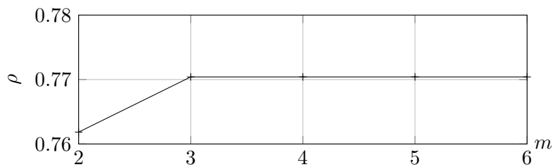
Figure 6.14.: Spectral radii of the m -grid error propagator with a single pre-smoothing iteration of Kaczmarz.
