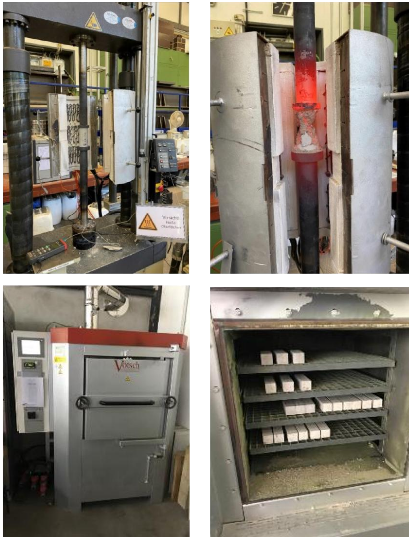
Figure 3.7 Heating systems used for the measurement of the hot compressive strength (up) and the cyclic thermal loading regime for the investigation of the residual compressive strength
