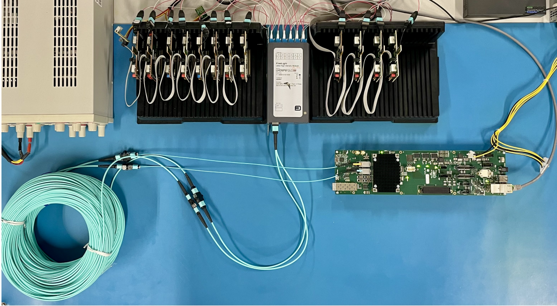
Figure 7.1: Benchmark study test setup comprising one EMP connected to 12 EMCIs.
