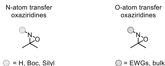
Figure 3.2 Reactivity patterns of oxaziridines exhibiting N- or O-atom transfer, dictated by the characteristics of the N-substituent.
