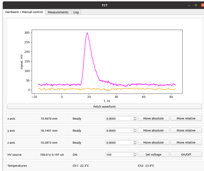
Figure 2.9: Control application for the Laserbox. The view with hardware monitoring and controls is presented. Signals, acquired from two adjacent strips of a sensor, are shown; the laser is set such that it deposits charge only in one strip (purple curve), so no signal is registered from the other strip (yellow curve).
