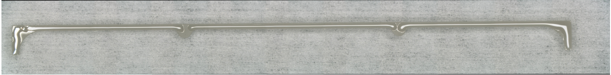
Figure 6.13: One spacer with slow glue dispensed on it. The automated procedure allows to reliably dispense a uniform line on a 1 mm wide spacer. Two gaps in the middle are left to apply the fast glue.
