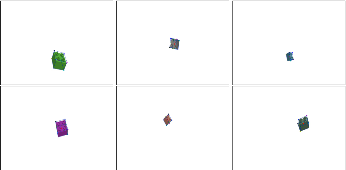
Figure 6.2 Bounding box predictions on the simulation test set. The perception module is able to accurately locate the object in the image.
