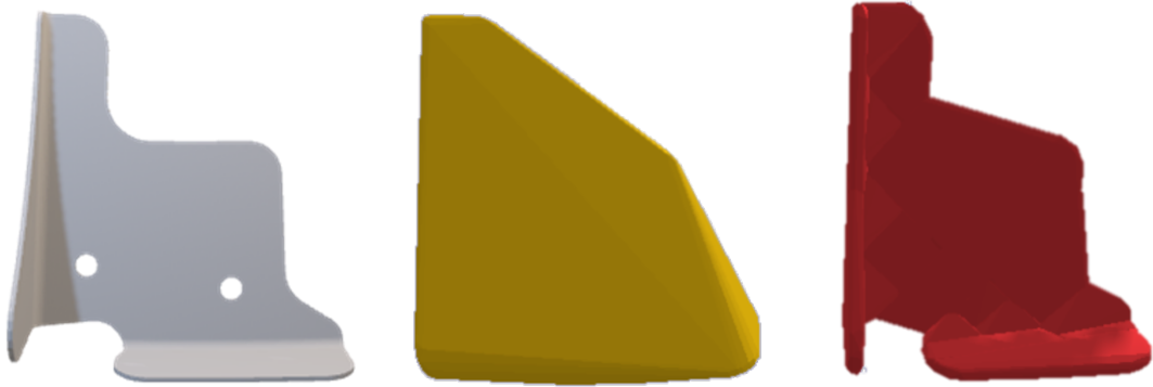
(a) The original mesh of the clip contains concave parts, which are not suitable for collision detection. (b) The convex hull approximation of the original mesh is too coarse and leads to collisions in simulation. (c) V-HACD provides a set of convex shapes, which are suitable for collision detection and precise enough for assembly.
