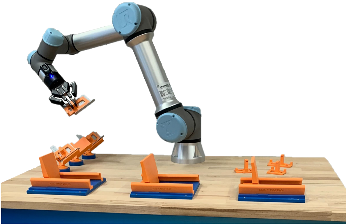
Figure 1.8 The clip assembly demonstrator consists of an UR5 industrial robot, clips and 3D-printed installation sites. The goal of the assembly task is to insert the clips into the shell structure.
