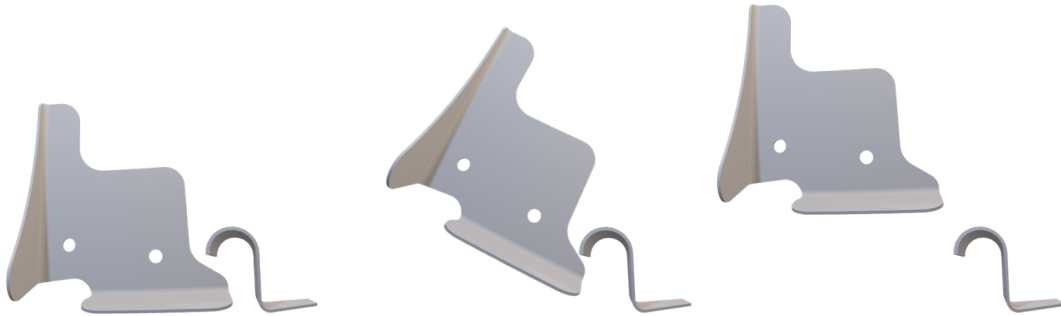
Figure 7.15 Reward hacking in the clip assembly environment. The agent is able to exploit the force constraint to move the clip out of the shell in a non-reversible manner.
