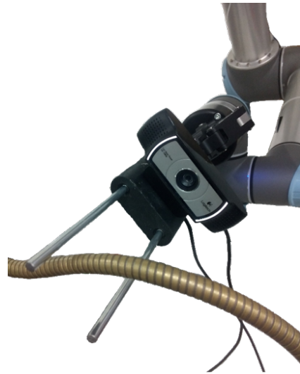
(b) The tool consists of two metal rods enclosing the wire and a camera for visual feedback. Taken from [114].
