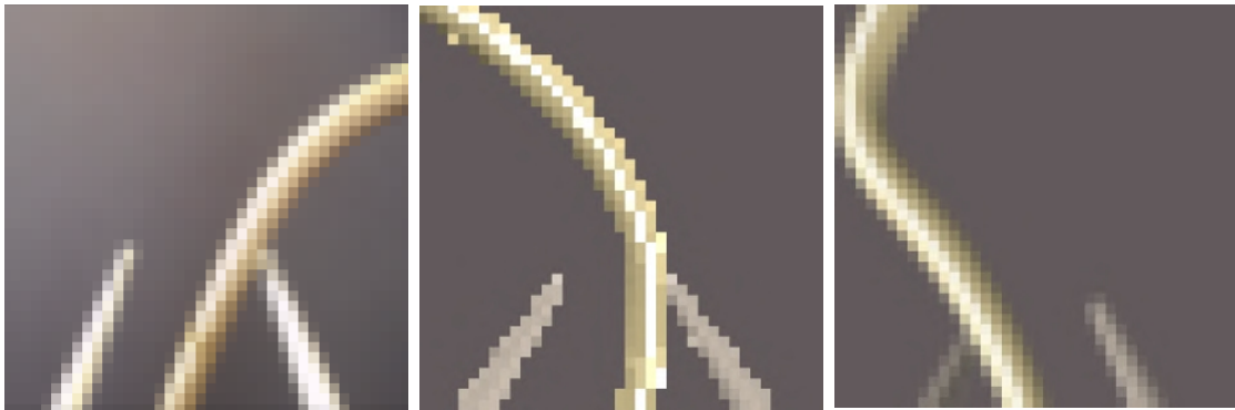
(a) Real-world image after down-sampling and interpolation. (b) Simulation image with direct down-sampling. (c) Downsampled simulation image. Taken from [154].
