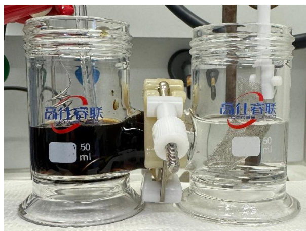
Figure 60. Example setup of an H-cell for lignin depolymerization. The cathode compartment (left) holds the lignin solution, working electrode, and reference electrode, facilitating reductive lignin depolymerization. The anode compartment (right) contains only the counter electrode and electrolyte. Gas formation at the anode indicates the electrochemical oxygen evolution reaction.
