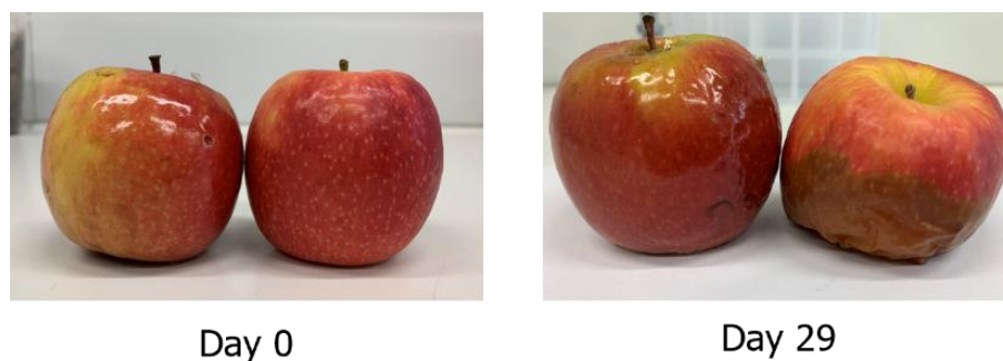
Figure 61. Preservation of an apple with a chitosan-DL coating (left) compared to an uncoated reference apple (right). Initially, both apples appeared fresh. After 29 days, the uncoated apple showed significant decomposition, whereas the coated apple exhibited minimal spoilage and retained its structural integrity.
