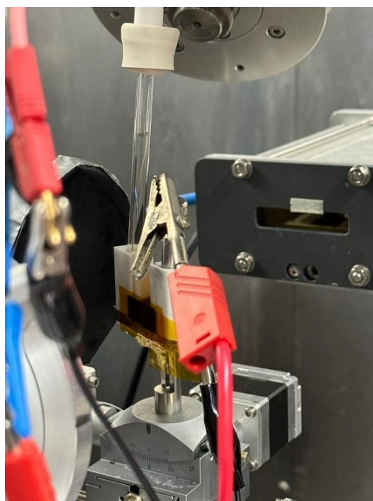
Figure S 51. Photograph of the in-operando experimental setup during synchrotron radiation measurements.
