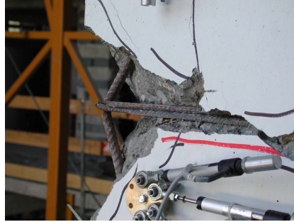
Figure 4.9: Pier A40: Buckling of longitudinal reinforcement at 3.5 m (PINTO ET AL , 2002)
