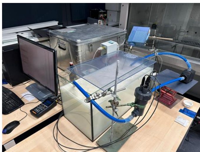
Figure 62: A setup with MWF in longtime experiments showing that measurements in highly concentrated emulsions are possible.
