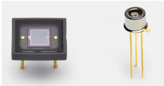
Figure 51: Left Hamamatsu photodiode S1227-33BQ and right Hamamatsu photodiode S16586. The form factor of the active area of the two diodes is entirely different. The active area of the one on the right is smaller, but it is more sensitive. These two models will be compared for further tests to determine a favourite for a photodiode module.
