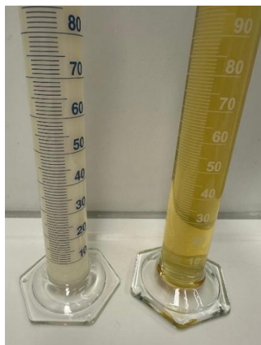
Figure 10: left is a 10% MWF emulsion based on several oils. The right one is a 10% MWF solution based on polyglycol. Both contain almost 20 ingredients with several aromatic components that are fluorescence active and ingredients that are reactive with chlorine dioxide.
