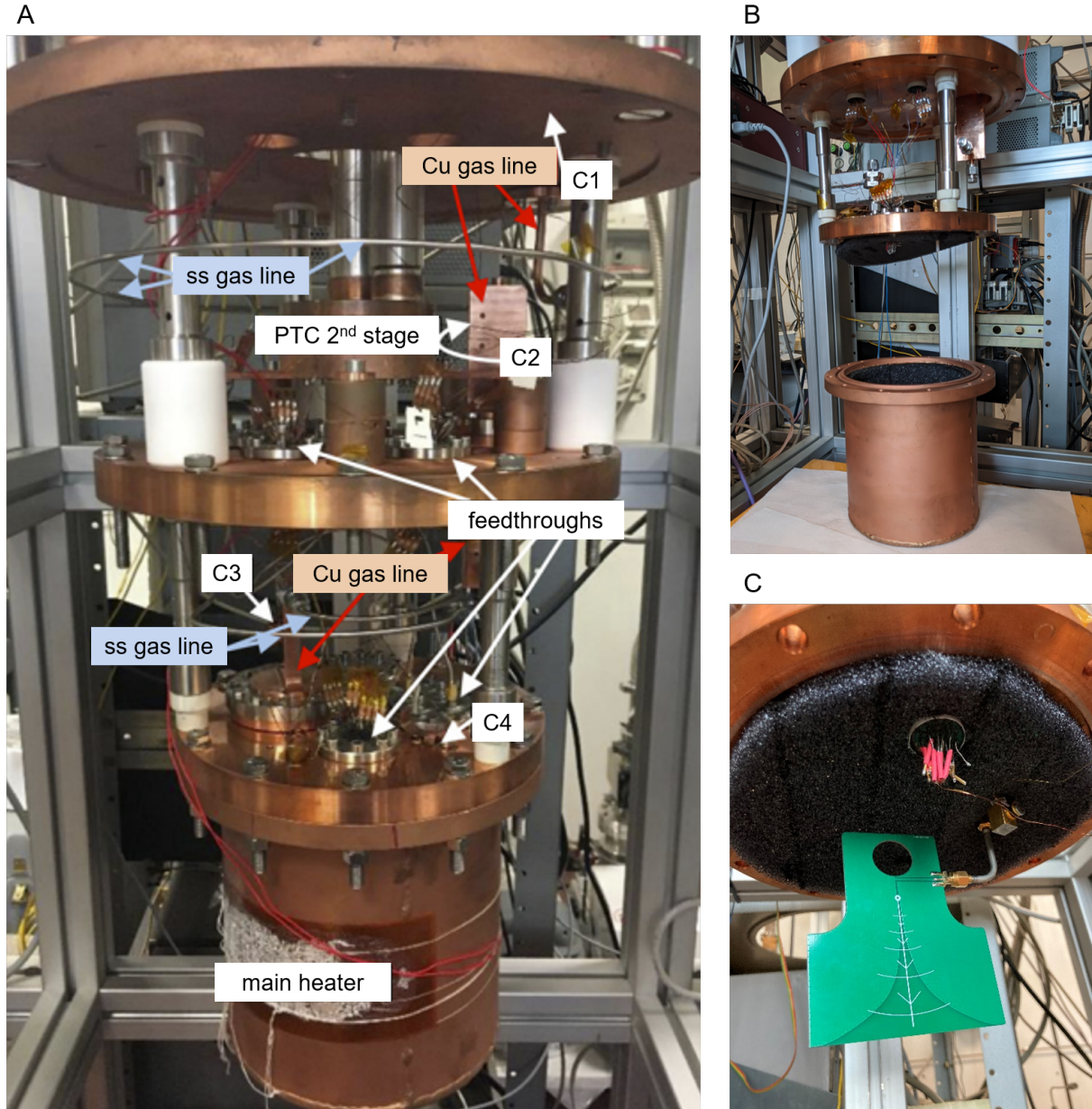
Figure 5.9: The apparatus is shown closed without the first cooling stage in A , (C1–C4) are Cernox® temperature sensors. For our measurement, there are additional temperature sensors within the cavity, behind the lining. The apparatus with an open cavity and monopole antenna in B , and open with a switched antenna-resistor position and a Vivaldi antenna in C . Fig. 5.9 a) has been adapted from [133, Fig. 4].
