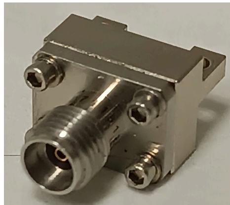
Figure 4.6: Image of the solderless 2.92 mm connector. The connector is to be screwed on the PCB with a support metal plate on the bottom side of the PCB.
