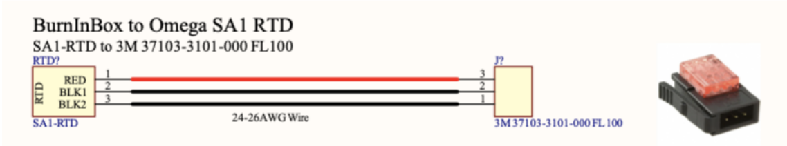
Figure A.1: RTD cabling scheme for the Burn-in box.
