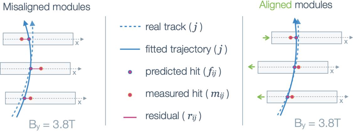
Figure 6.2: Schematic representation of a fitted trajectory (solid blue) with misaligned modules on the left and aligned modules on the right. The true trajectory of the charged particle is represented by a dashed blue line, while the predicted and measured hits are depicted as blue-red and orange-red dots, respectively. The residuals between these two types of hits are shown as solid red lines. Figure taken from [174].
