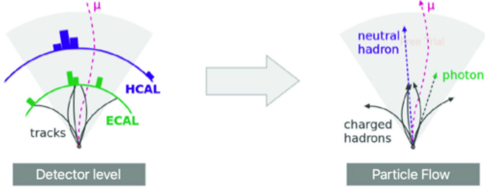
Figure 2.9: The Particle Flow algorithm achieves a full event reconstruction by identifying and reconstructing all final-state particles, including photons, electrons, muons, charged hadrons, and neutral hadrons. Figure taken from [115].
