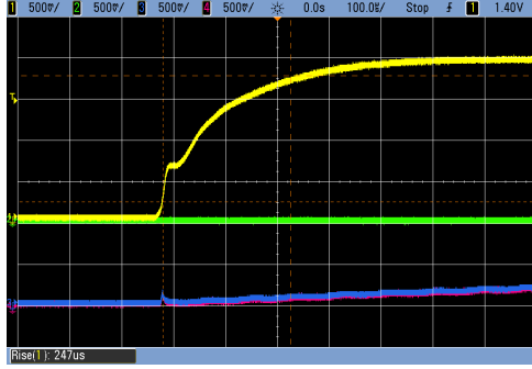
(a) Powering ON VCANA (0 to 2.0 V) while CANB is OFF, No load connected, Time/div=100 \mu s/div.
