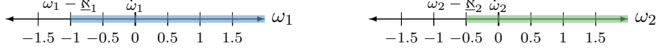
Figure 6.3. Illustration of the half closed feasible intervals for two weights if only lower IFBs, i.e., IFDs \underline{\aleph}_i , are used with \hat{\omega}_i = 0 \forall i = 1, \dots, N .
