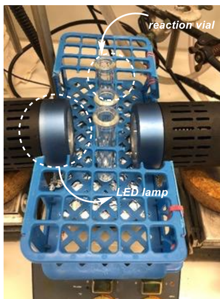
Figure 1: set-up using two blue LEDs (32 W, \lambda_{\max} = 440 nm) for reaction at 60 °C.
