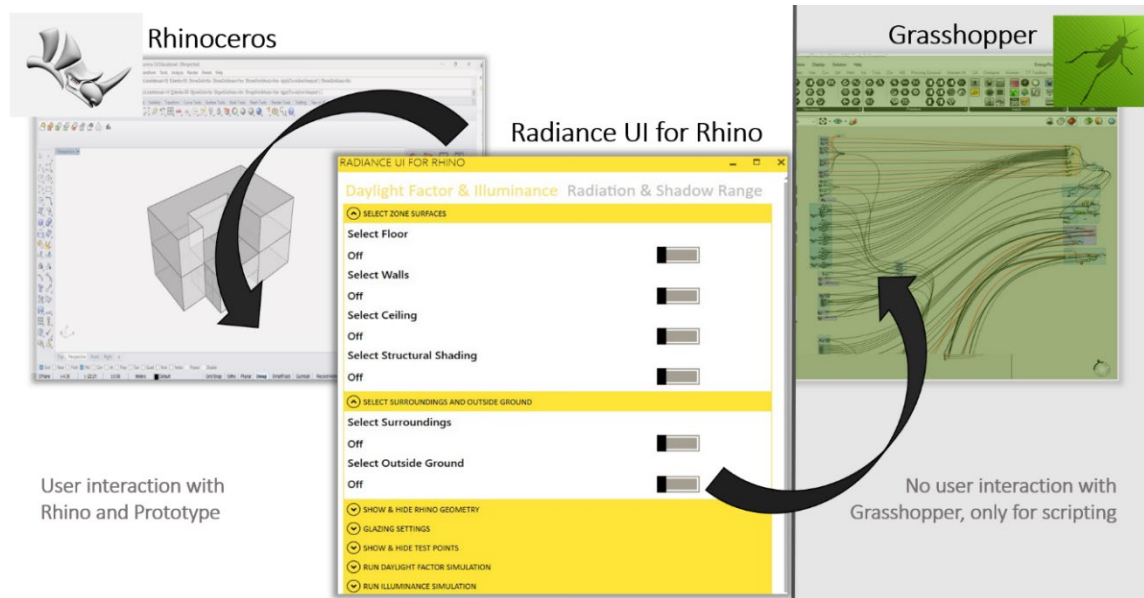
Figure 4. 8: Data flow via the “Radiance UI for Rhino” prototype and user interactions.
