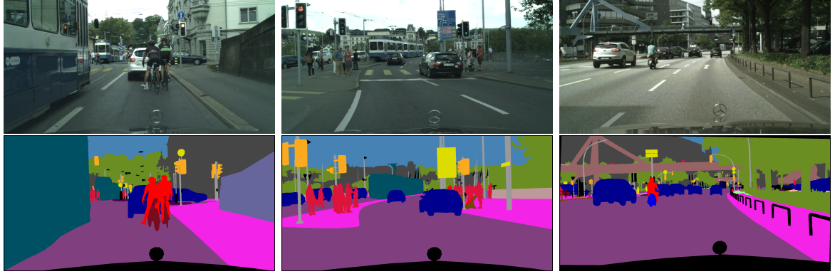
Figure 4.3: Example images from the Cityscapes dataset (first row) and their corresponding ground truth semantic segmentation masks (second row).
