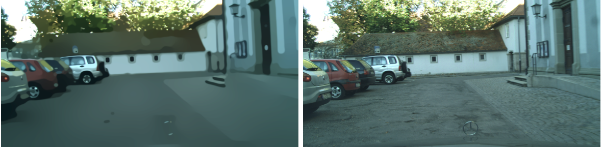
Figure 5.3: Image diffused by EED (left) and original image (right). The texture is smoothed along the edges but only slightly across them.
