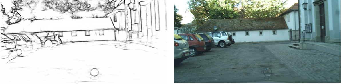
Figure 5.4: HED (left) and original image (right). The shape defining edges are preserved by HED whereas the finer texture defining edges are removed.
