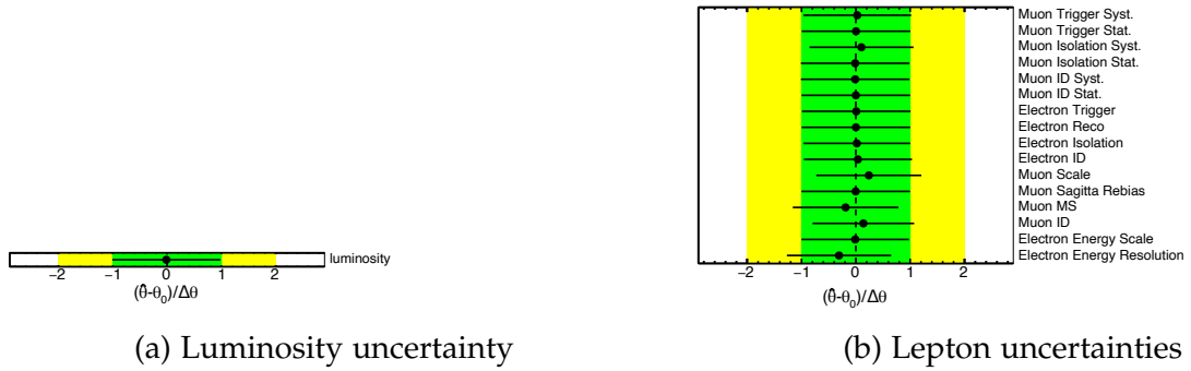
Figure 9.10.: ML estimators and their uncertainties for the nuisance parameters describing luminosity uncertainty in the left plot and lepton uncertainties in the right plot.
