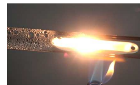
Fig. 1: magnesium burns in water vapour
