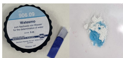
Fig. 2: White copper sulfate as a detecting agent for water.
