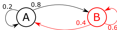
Figure A.12.: Transition diagram of a Markov Chain with two states showing the transition probabilities.
