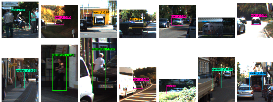
Figure 4.5: Examples of predicted bounding boxes with a true IoU = 0 but with high meta classification probabilities. These examples predicted by the YoloV3 network are counted as FPs as there is no corresponding ground truth available. Our prediction quality estimates signal with very high IoU values, that an object is present. The predictions, and therefore the data to train and evaluate gradient boosting, are obtained by the YoloV3 network applied to the KITTI dataset.
