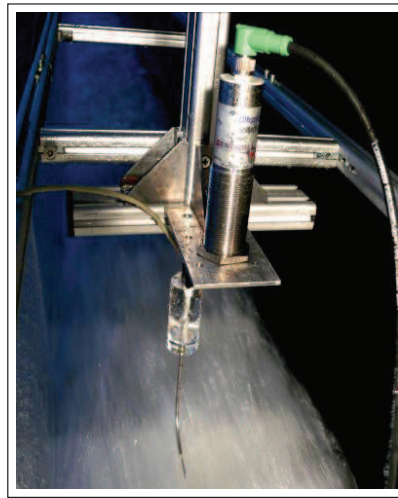
Figure 6.3.2: Ultrasonic sensor for determination of air-water mixture depth (note: double-tip conductivity probe below during measurement)
