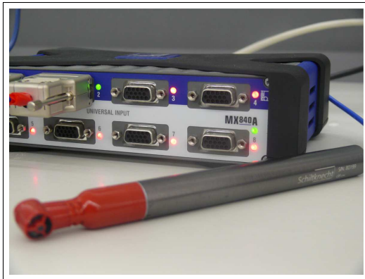
(A) Propeller anemometer plugged to an universal amplifier
