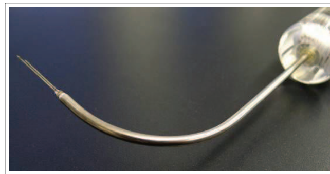
Figure 6.3.1: Double-tip conductivity probe for determination of air concentration and flow velocity (note: 2 electrodes with a distance of 5.1 mm in flow direction and 1 mm in cross-direction)
