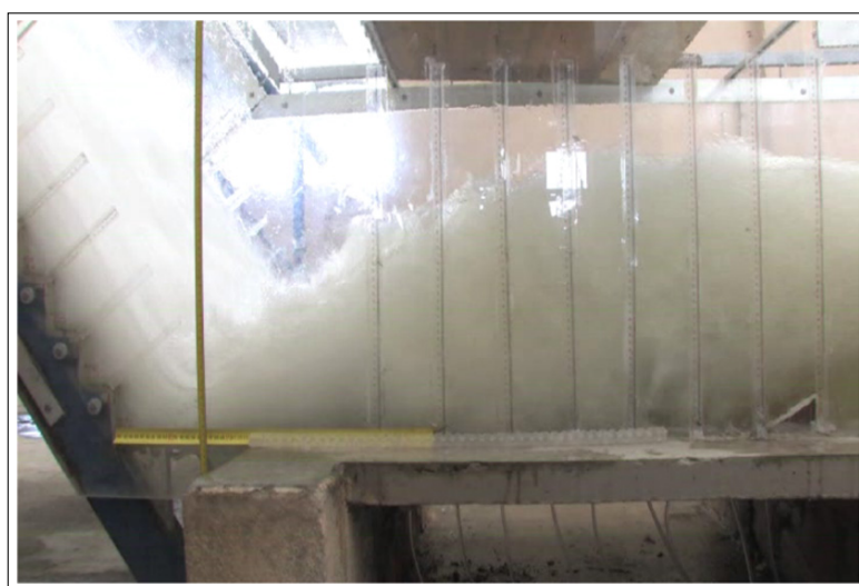
Figure 2.1.2: Model investigation on stilling basin performance downstream of a steep stepped spillway (BUNG ET AL. (2012)), channel width is 1 m to avoid model effects
