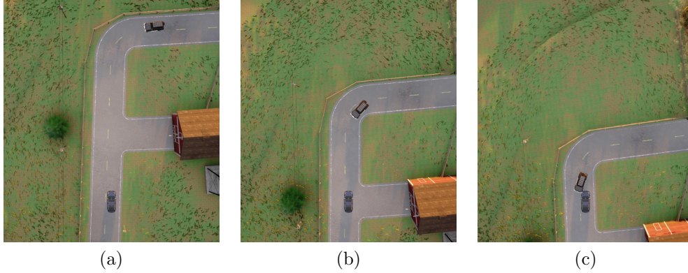
Figure 5.13: While driving too fast in a tight curve, one road user crossed the oncoming lane, resulting in a head-on collision between two road users. The consequence of a high goal and risk tolerance .
