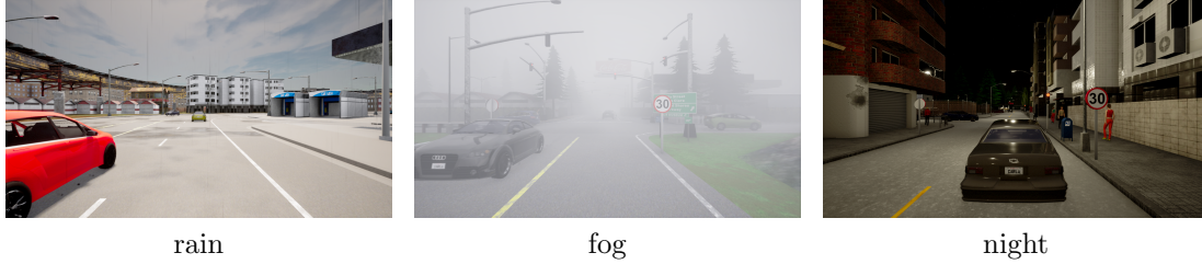
Figure 5.7: Overview of the used weather conditions. The grayish sky, falling water drops as well as water puddles on the road are characteristic for rain . In the case of fog , fine water droplets cover the image, and it is especially tough to see in depth. Night images are characterized by many dark areas, with streetlights and vehicle lights illuminating the scenes.
