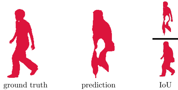
Figure 2.12: By means of the IoU for semantic segmentation, ground truth and prediction are compared with each other in such a way that the intersection of both is divided by the union.
