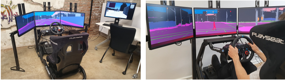
Figure 3.10: The fully assembled simulator with control center including peripheral devices and a monitor. The simulator can be used for demonstration purposes by driving freely in the virtual world of CARLA with support of a control unit and 3 monitors.
