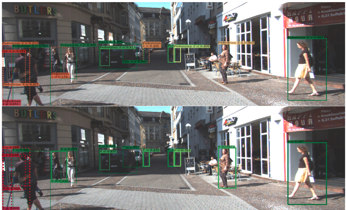
Figure 3.1: Object detection in a street scene. Top : DNN Score \hat{s} . Bottom : Meta classification confidence \hat{t} involving gradient features. Dashed boxes here indicate the discarding at any confidence threshold in [0.3, 0.85] . The top image contains FNs which are not separable from correctly discarded boxes based on the score (lower threshold would lead to FPs). In the bottom image, those \hat{s} -FNs are assigned higher confidences and there is a large range of thresholds with no FPs.
