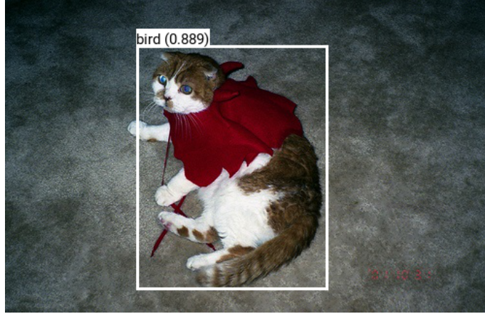
Figure 2.9: Prediction error of an object detection model (YOLOv3 [39]) on a previously unseen test sample of the Pascal VOC [38] dataset. While the localization of the predicted box is only slightly off, the predicted class is “bird” instead of “cat”. The number 0.889 in parentheses indicates the objectness score of the prediction, i.e., the overall confidence of the bounding box containing an object.
