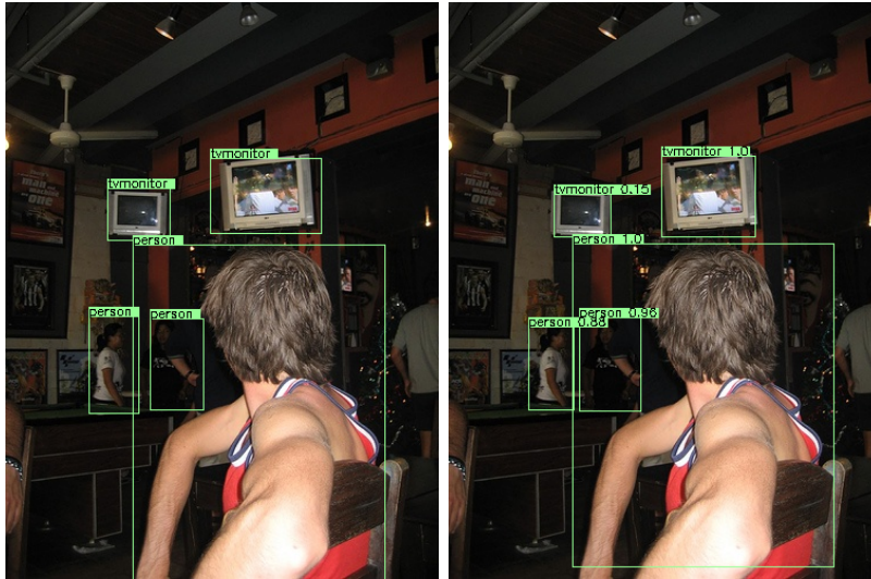
Figure 2.13: Object detection ground truth annotation ( left ) and prediction ( right ). The base image is taken from the Pascal VOC [38] 2007 test dataset. The prediction was produced by the YOLOv3 model with Darknet53 backbone used in the investigations in chapter 3. The ground truth consists of bounding box localization and category. Meanwhile, the final prediction has localization, assigned category and confidence score assigned. Usually, the category is determined from a predicted probability distribution.
