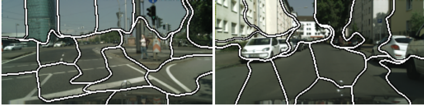
Fig. 2.5: Two randomly selected images from the Cityscapes dataset [18], segmented by the sparsity based SLIC superpixel algorithm [47]. The very rough semantic properties of the superpixels demonstrate the strength of the sparsity assumption in natural images.
