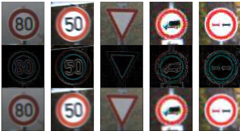
Fig. 3.7: A visualisation of randomly selected images from the GTSRB [130] dataset as: Top: the original images. Middle: the respective high-passed version. Bottom: The respective low-passed version.
