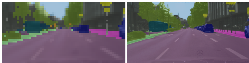
(a) Semantic segmentation at the smallest resolution of the model of [50] (b) Semantic segmentation at the full input resolution
