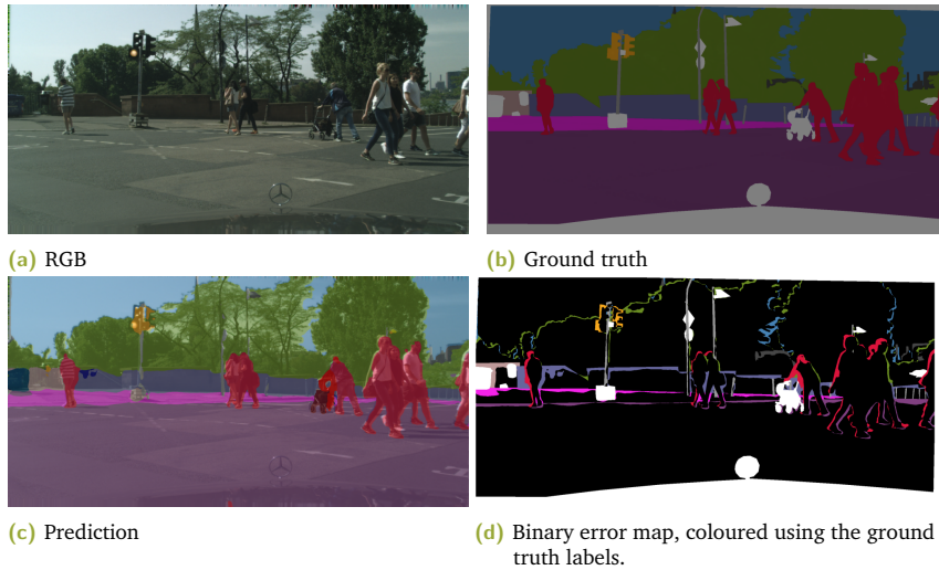
Fig. 2.9: A visualisation of the typical errors seen in semantic segmentation models. Notice how the mis-classifications, all not black pixels in (d), are concentrated around the borders while the inner parts are mostly well segmented. Visualisation created using the ‘FCN8’ model, trained on the Cityscapes dataset [18].
