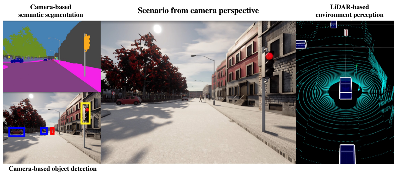
Figure 1.1: Environment perception of an intelligent vehicle using different sensors and AI-based perception systems (simulated example) 1 . In this work, we focus on the camera-based environment perception with focus on the object detection task.
