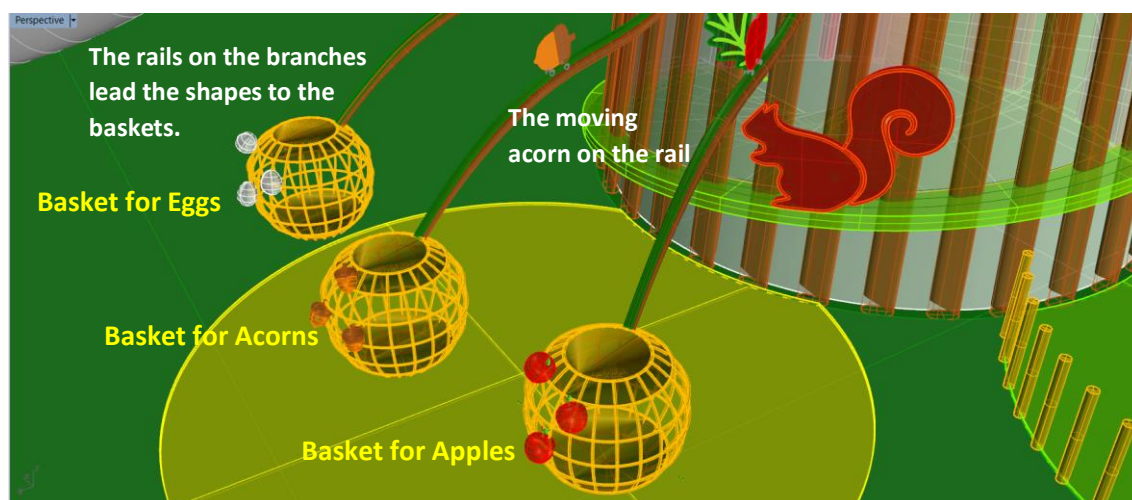
Figure 13-19: The moving shapes slide down on the rails spirally around the tree and finally fall in the baskets hung at the end of branches. The rails extend on the branches and lead the shapes to their baskets. Designer: Author.
