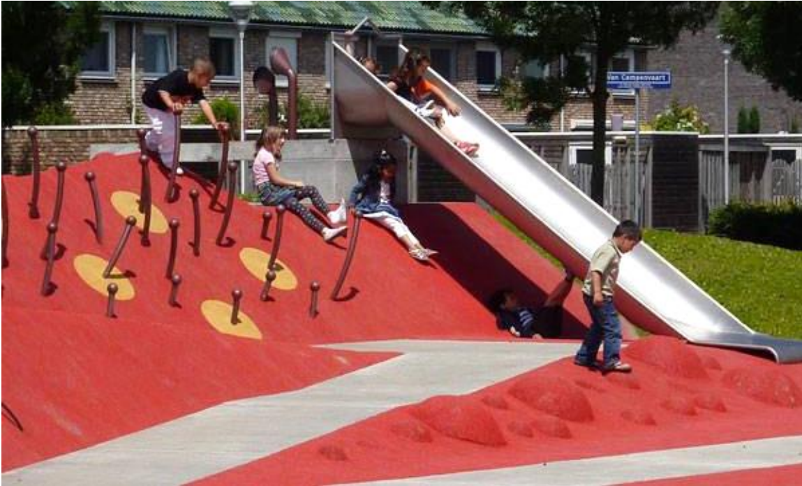
Figure 5-18: An embankment slide; installing the slide on a sloping surface with low slope and low height provides access for children with disabilities. Design: Carve.
