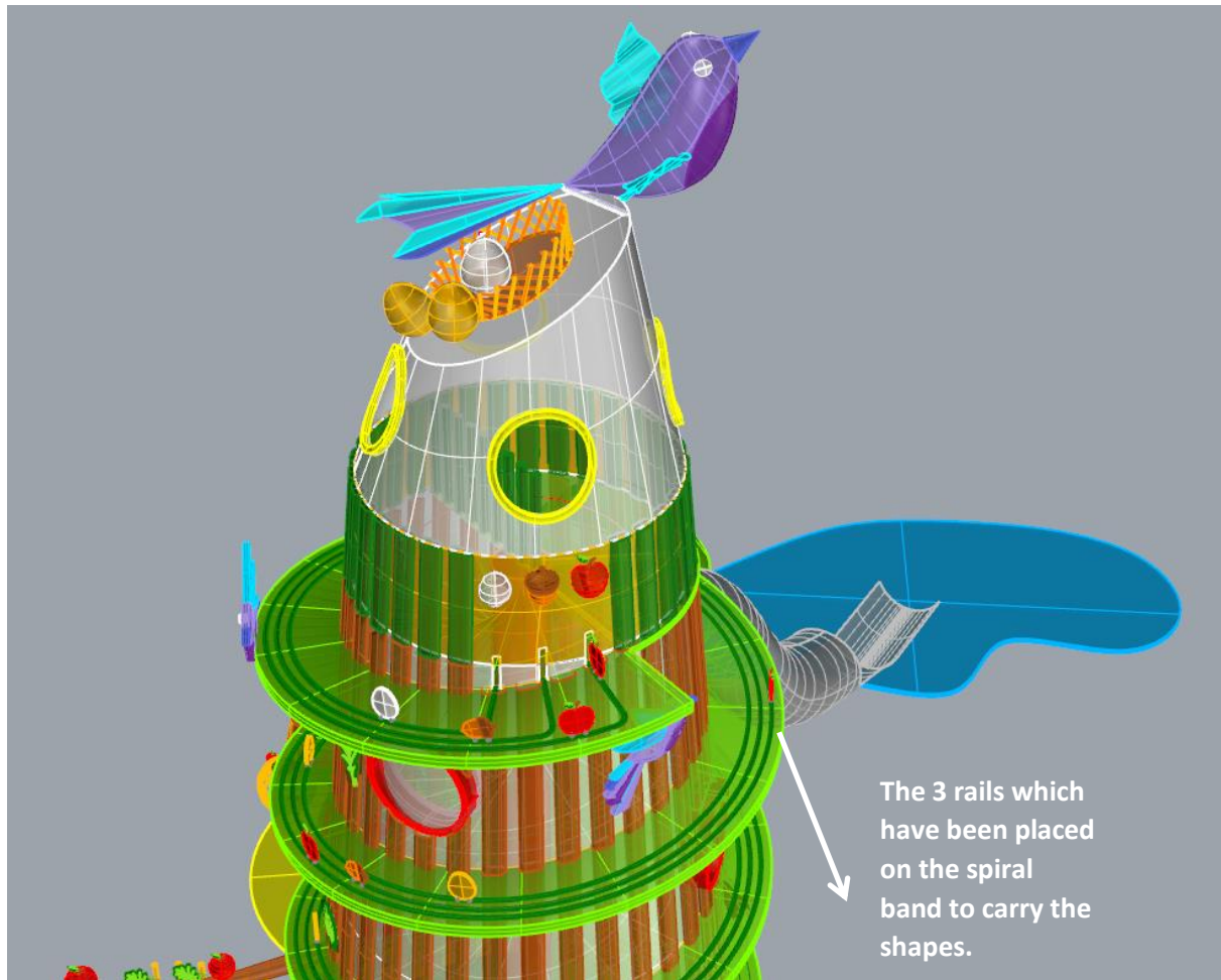
Figure 13-11: The upper part of the “Tree of Adventure” (also see the photos of this play structure/zone in Appendix 8 on the Attached CD).
