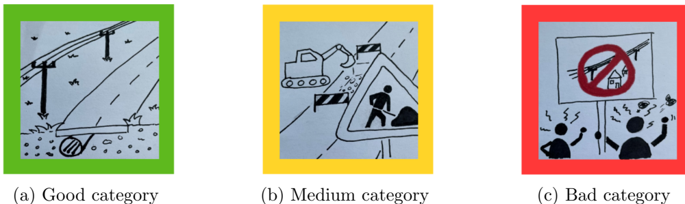
Figure 4.1.: Illustration of different edge or road categories for building new power lines or telephone cables.
