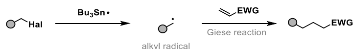
Figure 9. Giese reaction of alkyl radicals generated by the use tin hydrides and alkyl halides.
