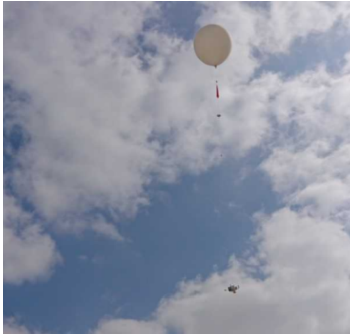
Figure 3.2: Weather balloon and payload as used during the measurements described in Chapter 4. The weather balloon with a parachute, unwinder and the large payload. The picture was taken shortly after the launch. The unwinder is slowly increasing the distance between the parachute and the payload, eventually reaching up to 60 m length.
