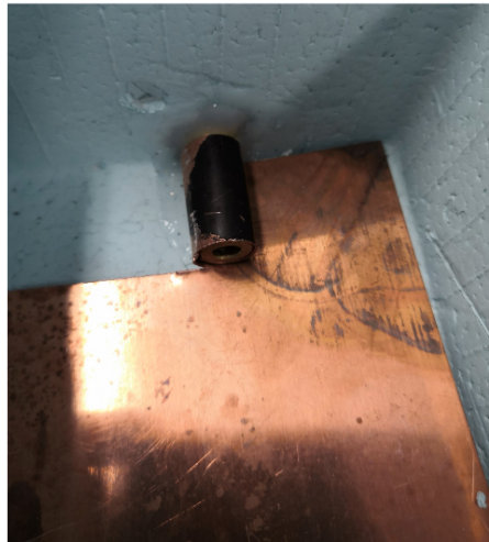
Figure 3.12: Picture of the copper plate mounted to the cold-finger of the CFH-CO 2 . with a minimum temperature of -116.18\text{ }^{\circ}\text{C} , 17.88\text{ }^{\circ}\text{C} less than inside the chamber. In order to improve the efficiency of the cooling agent, a copper plate was mounted at the CFH cold finger as shown in Fig. 3.12. Copper has a high heat conductivity of 386\text{ W m}^{-1}\text{ K}^{-1} at standard conditions which increases with decreasing temperatures (Carvil, 1993). The temperature heat conductivity dependence of copper is shown in Appendix B in Fig. B.1. Within the temperature range relevant for atmospheric balloon profiles, the thermal conductivity of copper slightly increases to 413\text{ W m}^{-1}\text{ K}^{-1} at -73\text{ }^{\circ}\text{C} . By enlarging the contact area of the cold finger to the cooling agent with the copper plate, the cooling efficiency is expected to increase. With this modified CFH a second test flight was performed. The results can be seen in the Fig. 3.13 and Fig. 3.14. As expected, the performance of this test flight shows improved cooling efficiency of the CFH-CO 2 . The temperature of both
