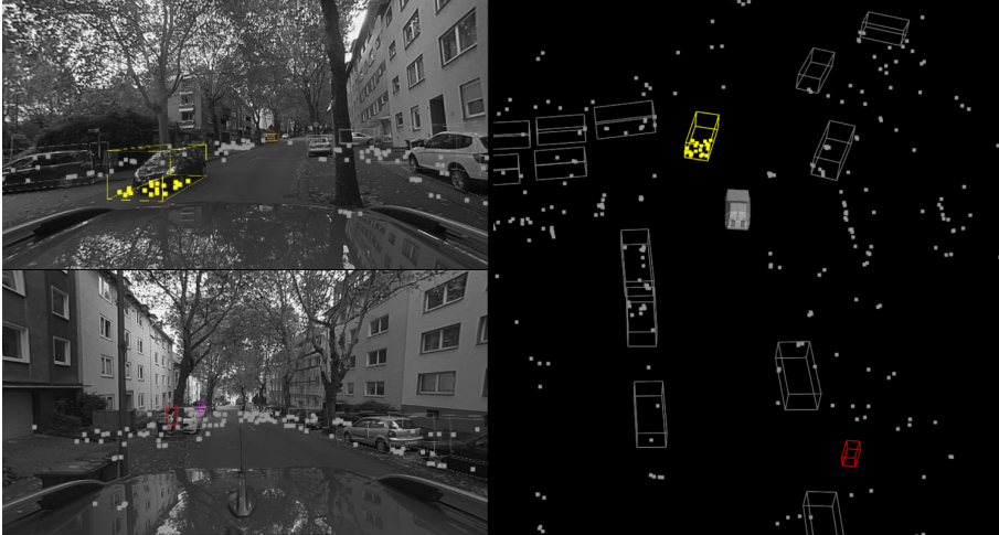
Figure A.3: Incoming moving vehicle correctly detected by the network. Points from all the other parked vehicles are classified as the negative class. The pedestrian on the rear does not have any associated reflection. Since it is occluded by a parked car, the sensor could not see this instance. Top-left: front camera. Bottom-left: rear camera. Right: 3D view.
