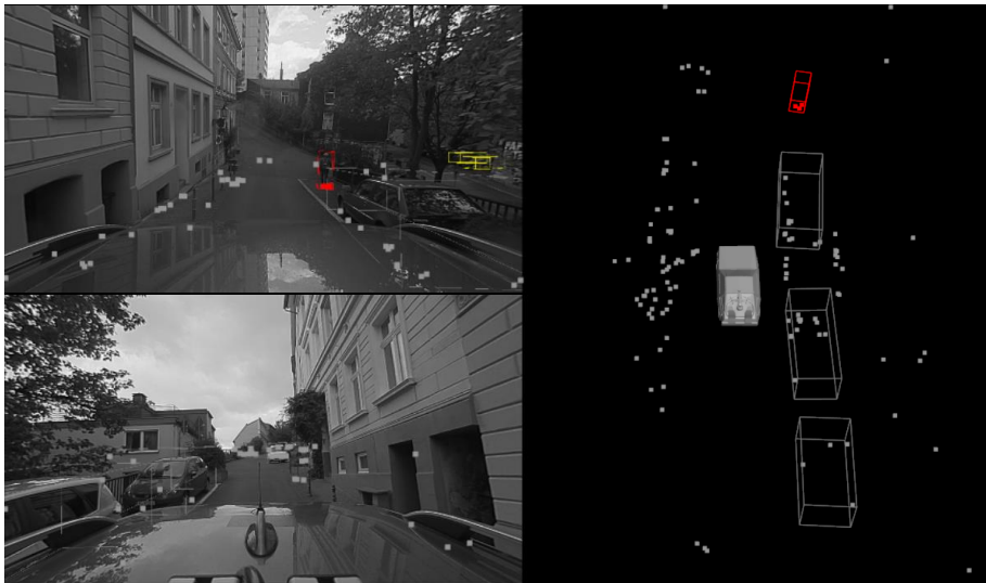
Figure A.6: A pedestrian in front of the ego-vehicle, near parked cars, correctly detected by the network. The rest of the scene is classified as static. Top-left: front camera. Bottom-left: rear camera. Right: 3D view.
