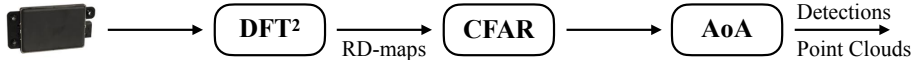
Figure 2.6: Overview of FMCW radar digital processing chain. The discretized signal is processed with two dimensional DFT (fast- and slow-time) to produce RD-maps. The CFAR algorithm detects target signals from noisy ones. Finally, an AoA algorithm extracts angular information to generate a point cloud of detections.
