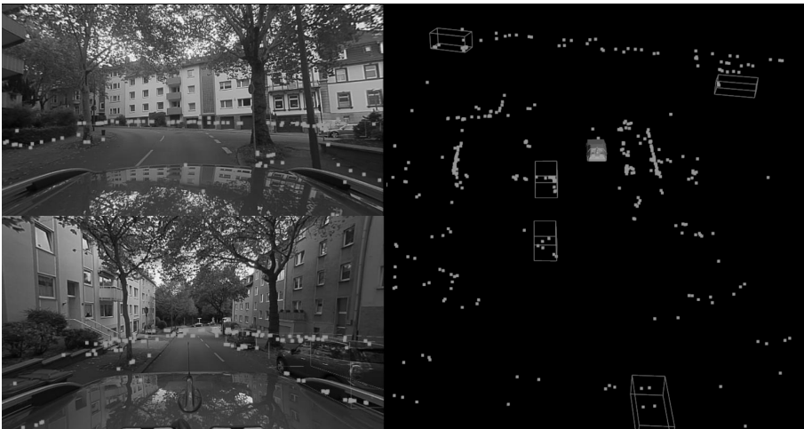
Figure A.4: The scene contains only static objects and the network can correctly predict the negative class for every point. Top-left: front camera. Bottom-left: rear camera. Right: 3D view.
