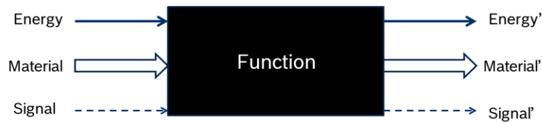
Figure 17 The Black-Box model of the function of a technical product [Pahl et al. 2007]
