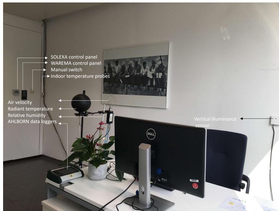
Figure 4.3: Locations of indoor sensors in the test room.
