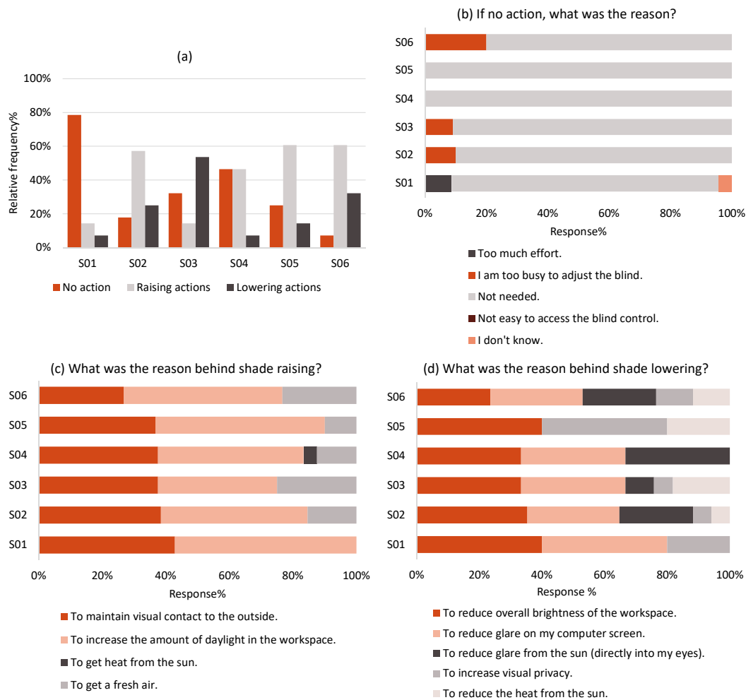
Figure 4.31: (a) User-shade override frequency (b) reasons behind no action (c) reasons behind shade raising (d) reasons behind shade lowering.
