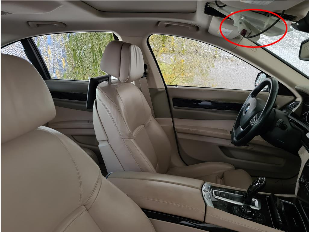
Figure 2.8: Example of the ToF camera location in one of the test cars. The camera is installed in the roof module of the car in such a way that it observes the front seats.
