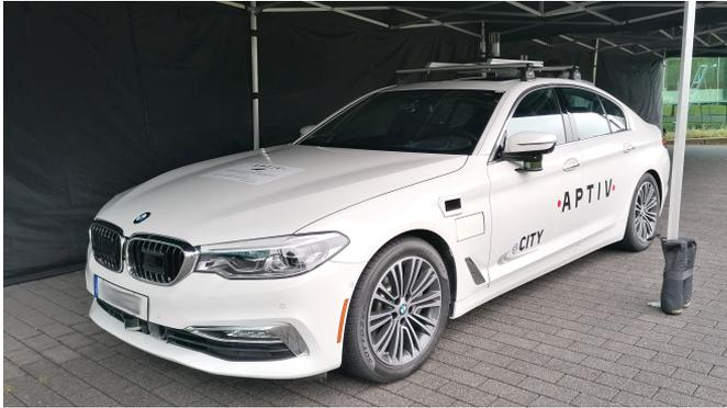
**Fig. 7.6.:** The car used for activities in the @City project. The main sensor, Hesai Pandora, can be seen mounted on the roof.
